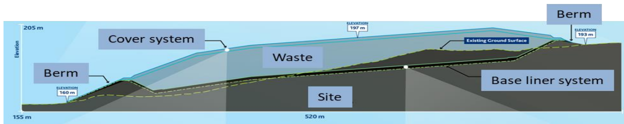
Figure 3-18 Cross Section of the Engineered Containment Mound
